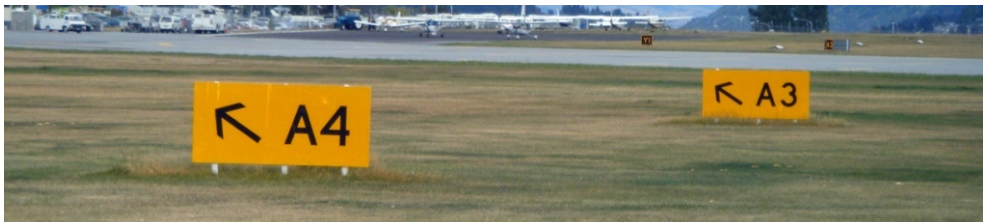
16-21 - Taxiway Direction Signs
